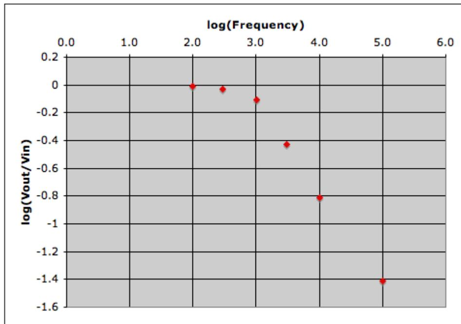
Figure 0.2: Bode Plot for a Low Pass Filter
