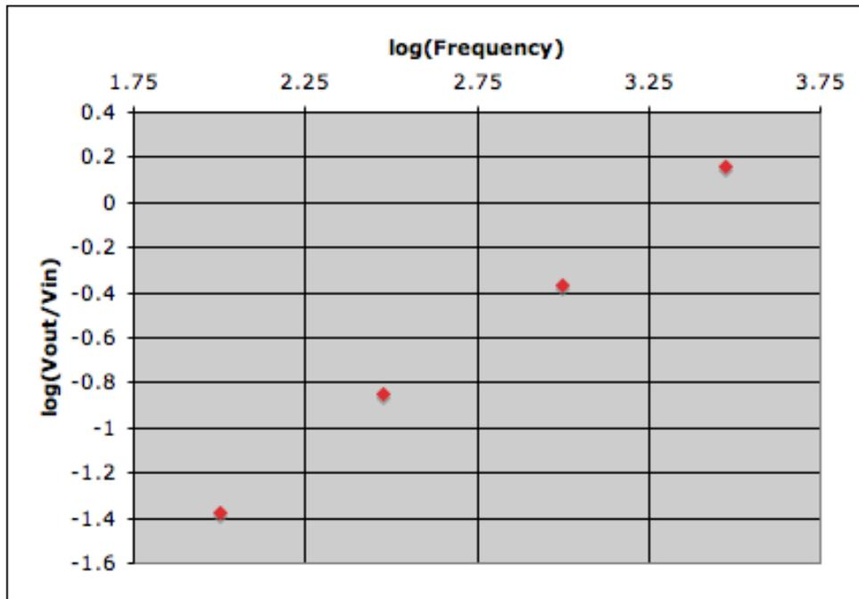
Figure 0.3: Bode Plot for a Differentiator
